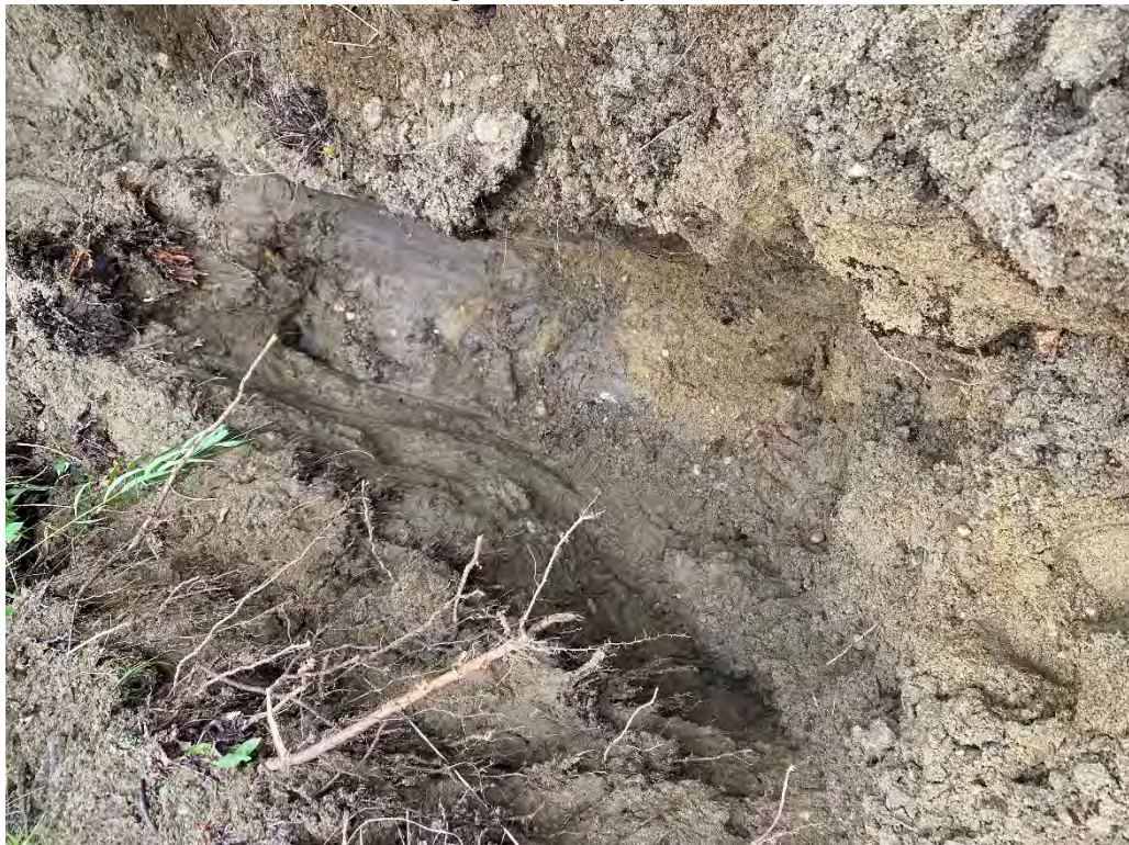
Photo 12: Soil with elevated PID readings in Test Pit TP3 was from gray soil layer. (July 15, 2021)
