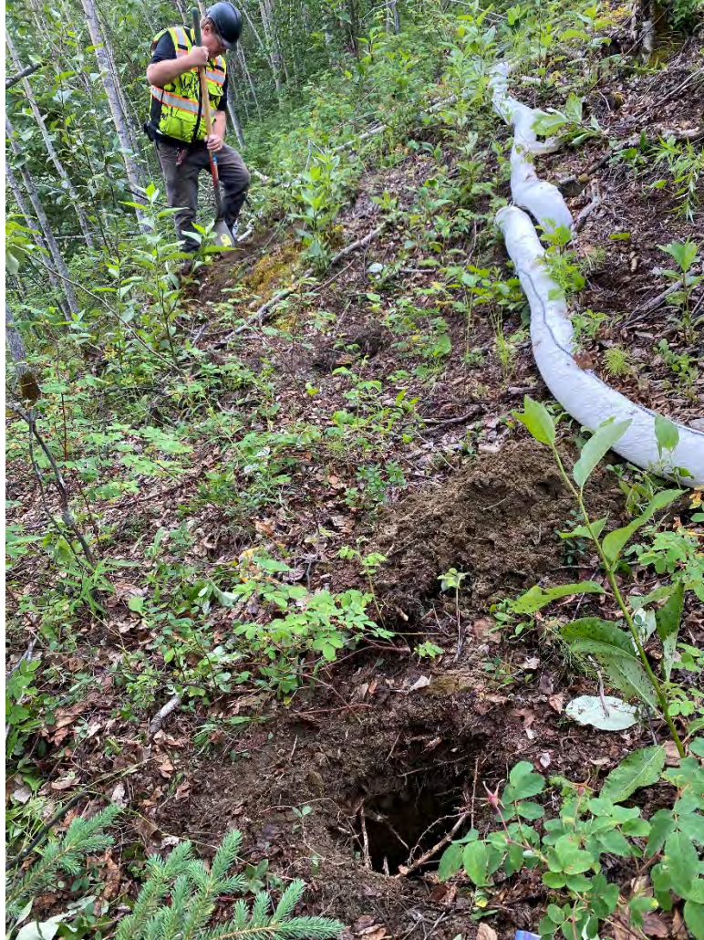
Photo 15: Advancing Test Pit TP7 and completed Test Pit TP8 in the foreground; looking southwest. (July 15, 2021)
