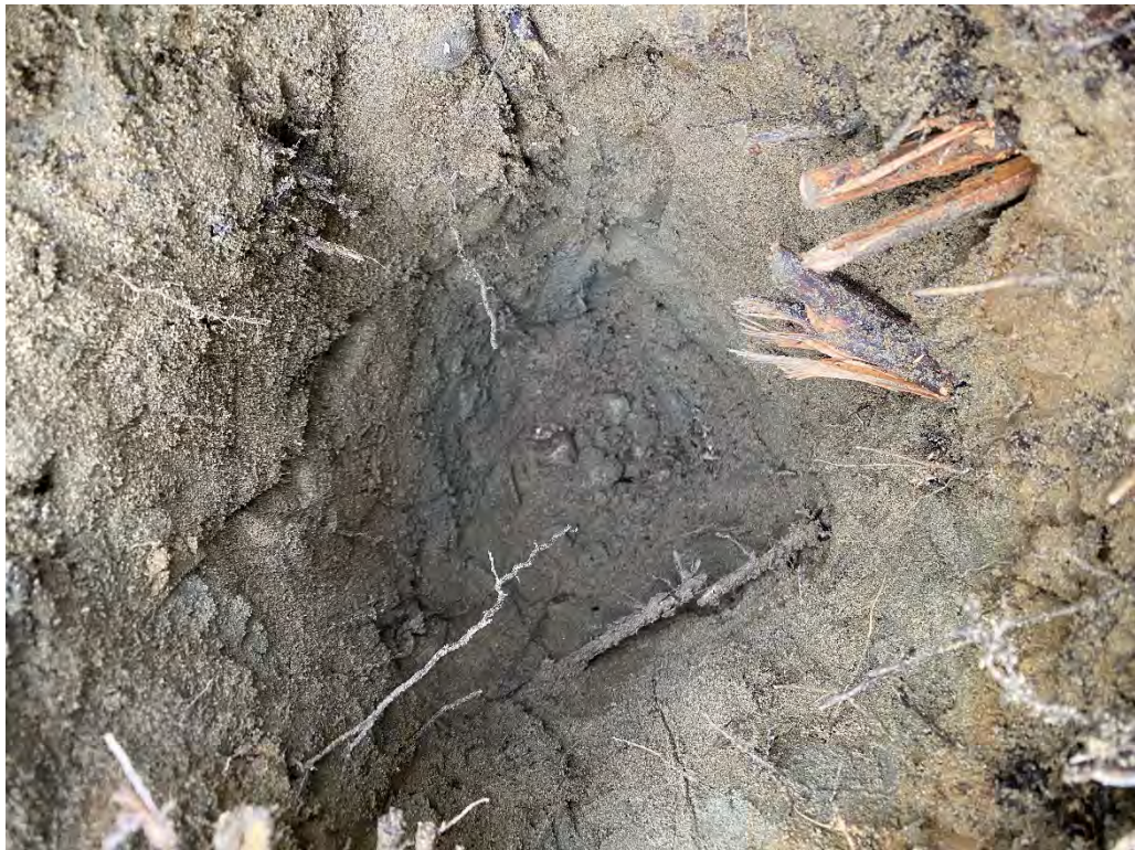
Photo 14: Gray silt layer in Test Pit TP7. (July 15, 2021)
