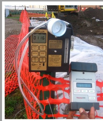
Figure 7: Air sampling device
