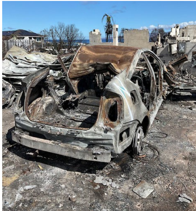
White lightning bolt painted over blue lightning bolt indicating that battery has been removed.
