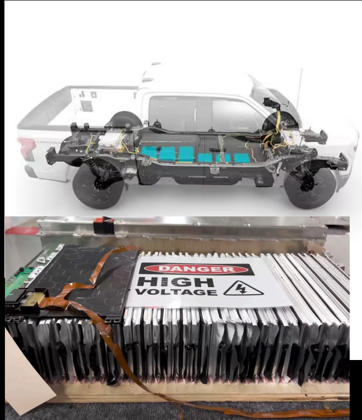
Ford Lightning Battery Pack Pouch Cells
