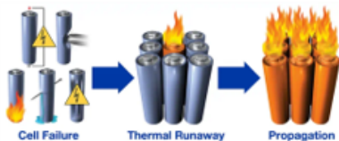
Figure 1: Diagram depicting a cascading thermal runaway event.
