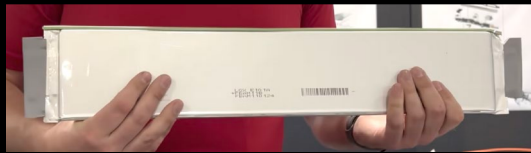
GM Battery Pack Pouch Cells
