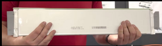
GM Battery Pack Pouch Cells
