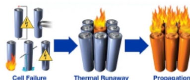
Figure 1: Diagram depicting a cascading thermal runaway event.
