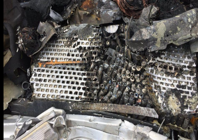
Tesla – Cylindrical Cell Batteries 18650 cell generation
