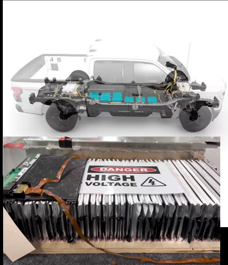
Ford Lightning Battery Pack Pouch Cells
